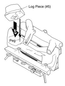
Figure 25 - Installing Log Piece (#5)
